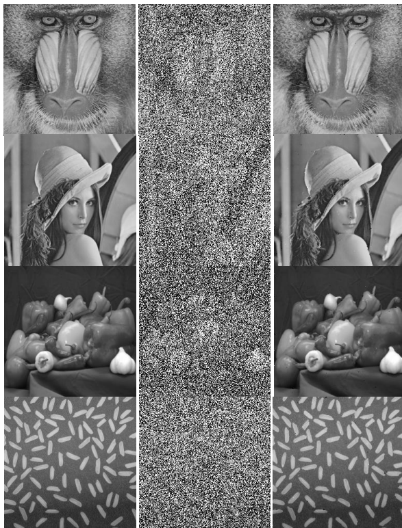
Fig.4 Performance of test images: First column represents original images, second column represents images corrupted with 70% of noise and third column represents images enhanced by proposed filter
