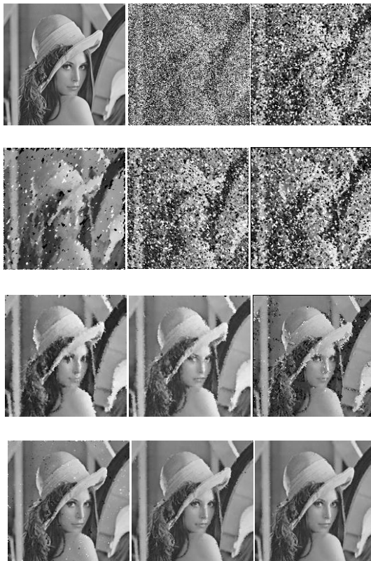
Fig.2 Subjective Performance comparison of proposed filter with other existing filters on test image Lena (a) Noise free images, (b) image corrupted by 70% impulse noise, (c) images restored by MF, (d) images restored by WMF, (e) images restored by CWMF, (f) images restored by TSMF, (g) images
