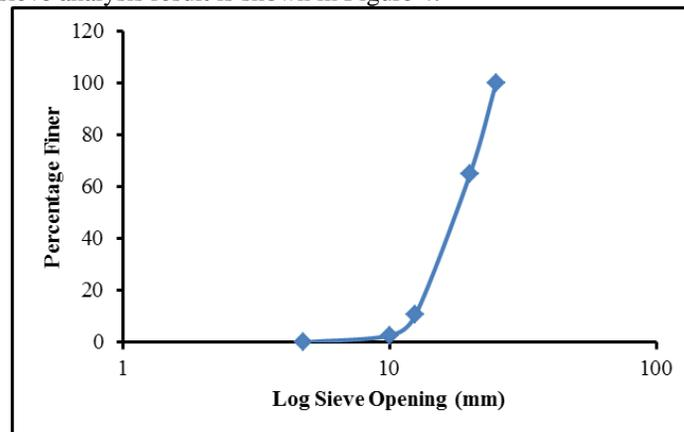
Figure 4: Particle size distribution of Coarse Aggregate
