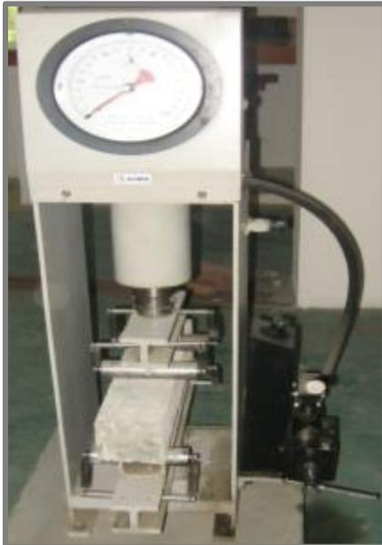
Figure 7: Flexural Strength Test
