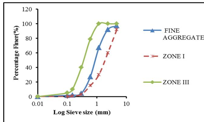
Figure 3: Particle size distribution of Fine Aggregate
