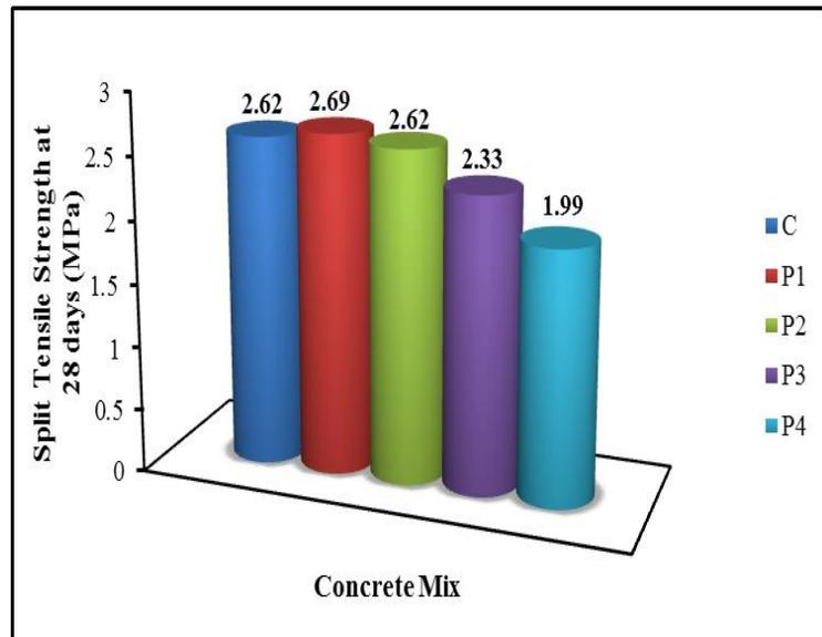
Figure 8: Variation of Split Tensile Strength
