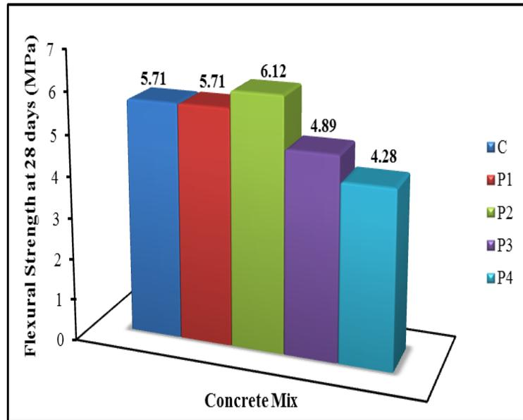
Figure 8: Variation of Flexural Strength
