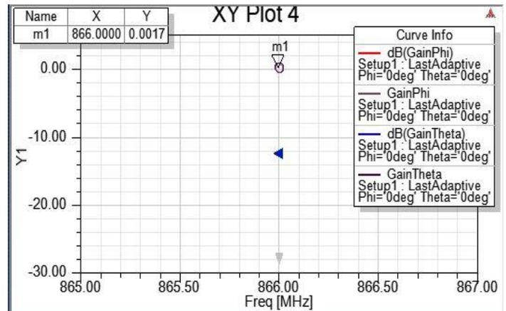
Figure 3.3 Overall gain of the MLA patch .A nearly 0 dBi gain is observed
