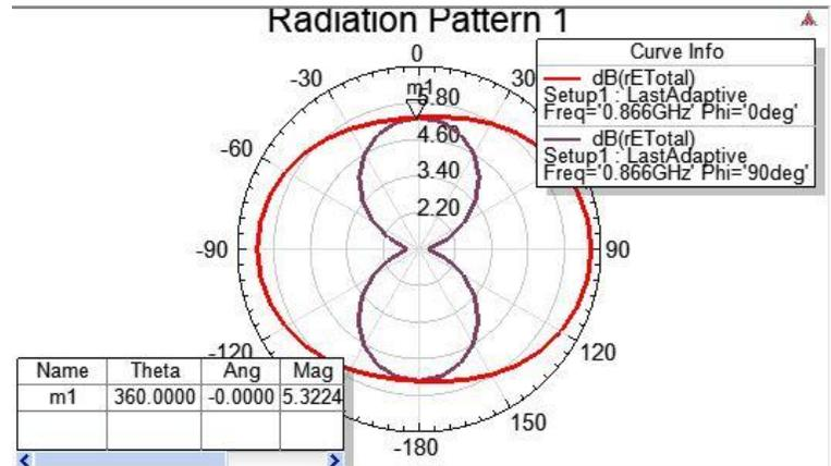
Figure 3.2 Radiation pattern of MLA Patch .An omnidirectional pattern is observed.
