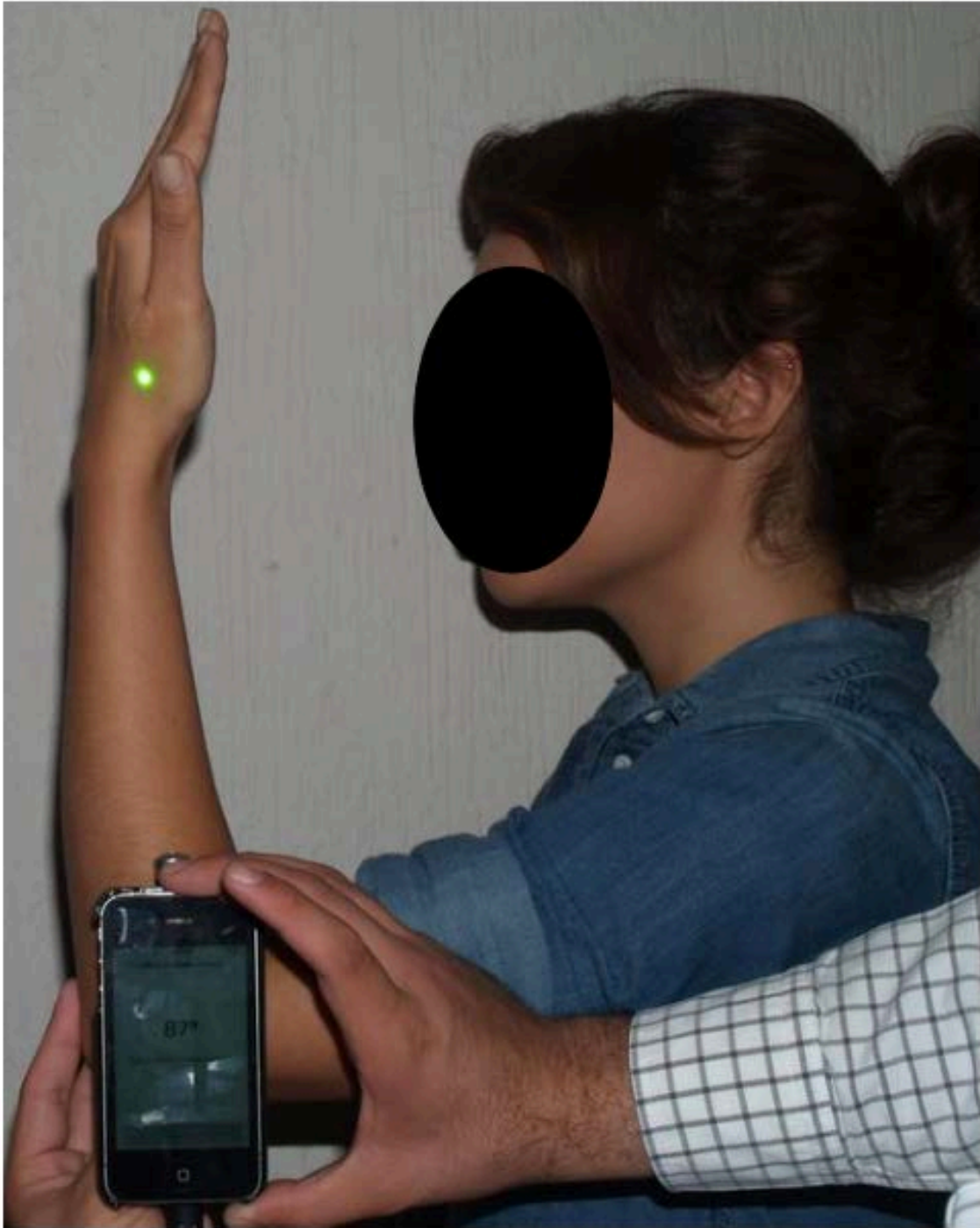
Appendix L: First generation laser goniometer. ROM of left elbow flexion 87° degrees.
