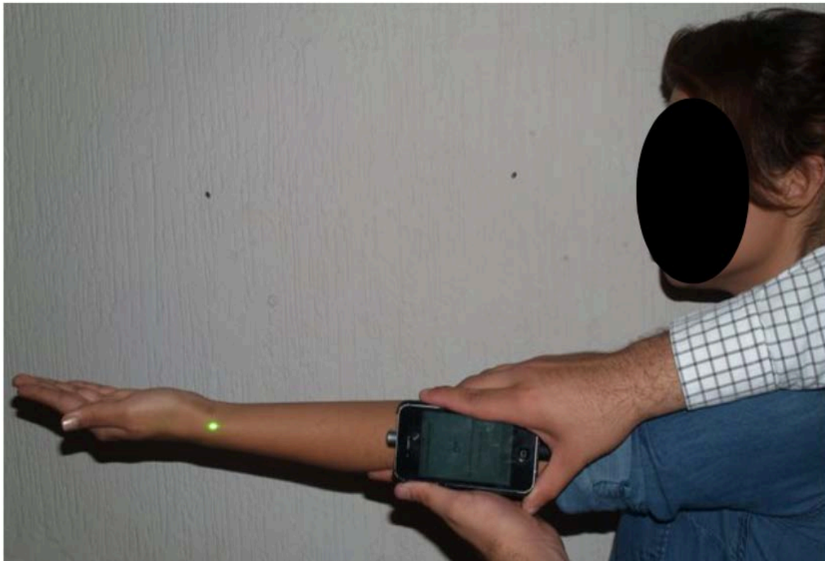
Appendix K: First generation laser goniometer. ROM of left elbow 0°. Zero starting position. The first generation laser goniometer was a 3D printed ABS plastic case that held a green laser pointer in place.
