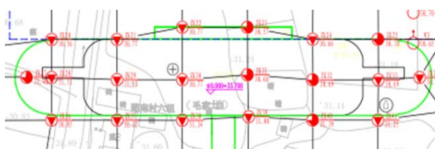
Figure 2.1. Exploration holes in the main building.
