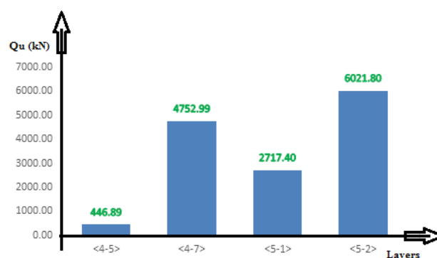
Chart 3.1. Layers x Qu by the method of Aoki and Velloso.
