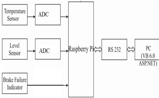
Fig 1.1 Block diagram
