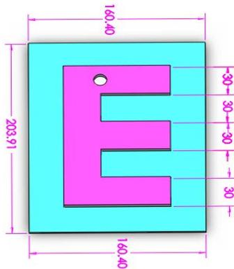
Figure 1: E-shaped printed antenna
