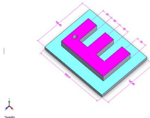
Figure 2; Isometric View of the E-shaped Patch Antenna
