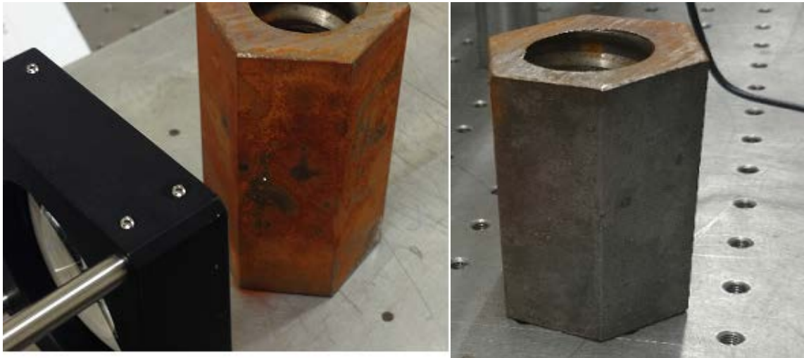
Fig 1. Mild Steel sample showing rust layer and regular surface sections
