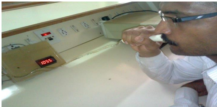
Fig 5.2: Technique for recording the maximum bite force
