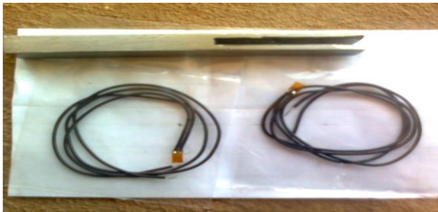
Fig2.1: Strain gauge with wire connection
