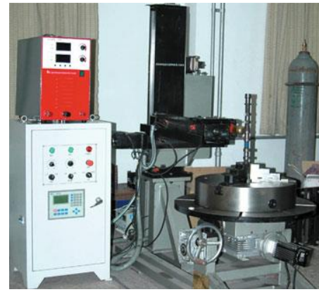
Figure 2.19 Self developed PTA forming remanufacturing system (zhu, 2013).
