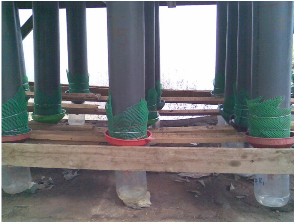
Figure: 1 Arrangement of Leaching column
