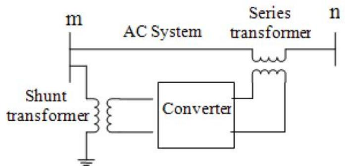
**Fig. 1 Schematic Diagram Of The Thyristor Controlled Phase Shifter**
