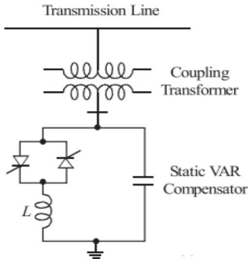
Fig. 6 SVC connected to a transmission line.
