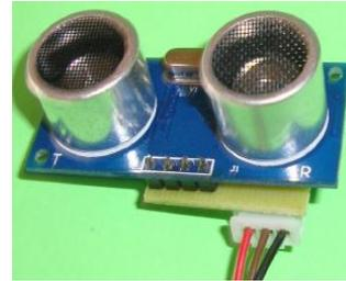
The ultrasonic sensor is utilized as substitute and the gesture is recognized in terms of different distances and the hand movements for various distance acts as gesture sign for control applications. The ultrasonic sensor output signal is fed to the microcontroller ATMEGA32 via the serial interface. A suitable embedded 'c' program is written the algorithm here, read the different hand gesture sign senses by the ultrasonic sensor and becomes different control operation.
