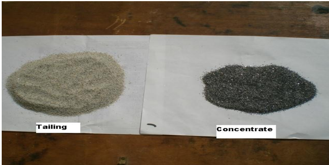
Plate II: Typical products of multi-gravity separation.
