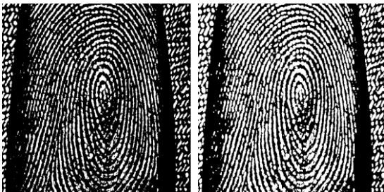
Figure 5: Binarized image (left) and wiener filter after binarization (right).
