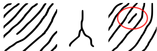
Figure 2: Minutiae features: Termination, bifurcation, short ridge.
