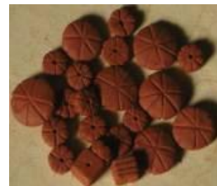
Figure 27, Terra sigillat made with soil of Baswa and applied on terracotta beads
