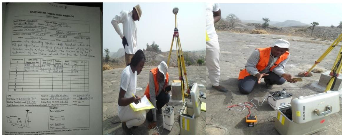
Plate 1. (a, b and c) shows the sample of the gravity data field sheet and the pictorial view of the gravimeter when the observation at Kwoi was in progress.
