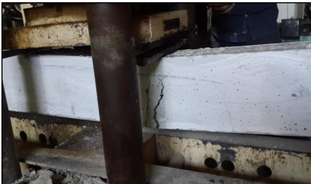
Figure 10: Cracks on the green bamboo reinforced beam sample
