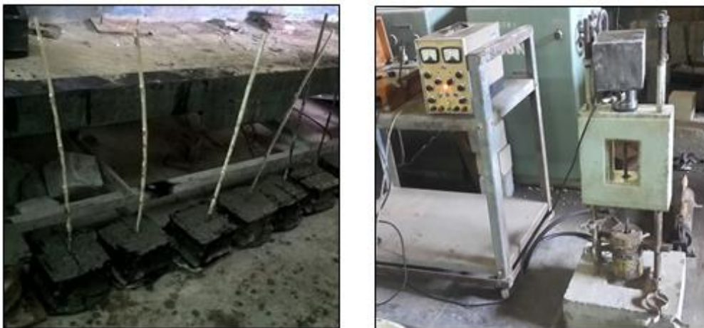
Figure 4: Pull out test samples and test setup
