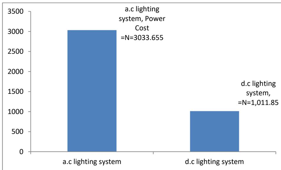
Figure 2: a.c lighting versus d.c lighting cost
