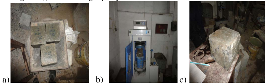
Figure 1 Concrete Samples during Compression. a) Sample after curing, b) Digital compression testing machine, c) Concrete Sample after failure.
