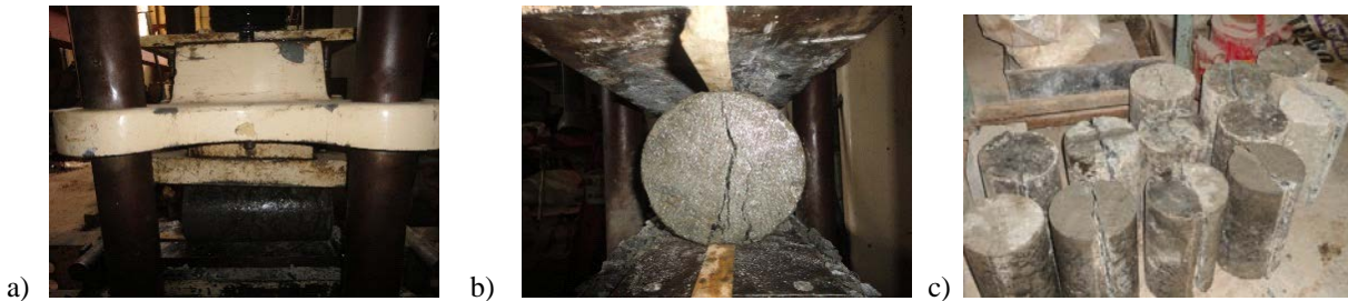
Figure 2 Samples in splitting tensile test, a) and b) Concrete Sample in the Universal Testing Machine, c) Concrete Samples at failure
