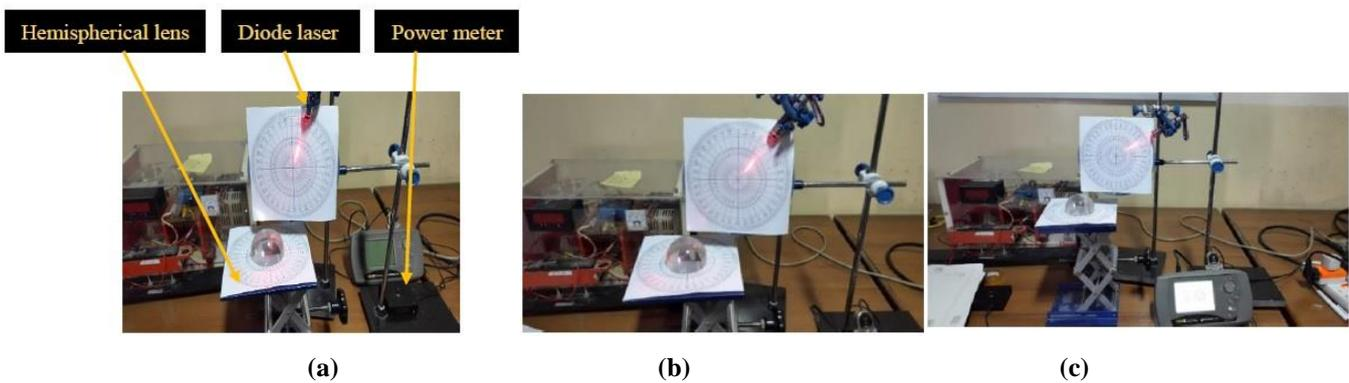
**Figure 3 a, b, c: Experimental setup of diode laser (Waveleight 632 nm) at different angle of incident to measure refractive index and reflectivity of the hemispherical lens.**
