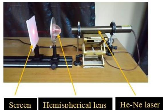
**Figure 2: Experimental setup using He-Ne laser to measure focal length of hemispherical lens**
