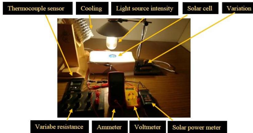
Figure 4: Experimental setup to measure output parameters of the used solar cell
