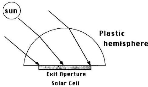
**Figure 1: Hemispherical lens that used to generate a concentration ratio of  $n^2$ [7].**
