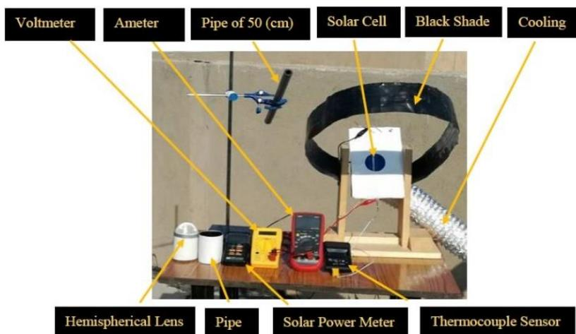
Figure 5: Experiment setup to measure and concentrate solar light component (W/m<sup>2</sup>) using the hemispherical lens.
