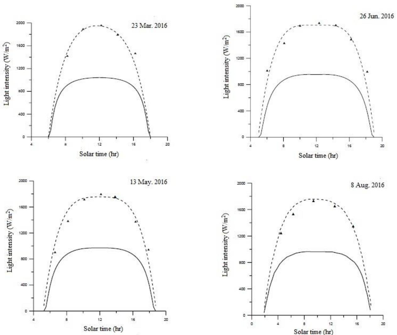
**Figure 8: Solar light intensity without lens (solid line) and with hemispherical lens (dashed line) that best fit experimental data (solid triangle) at 23 Mar., 13 May, 26 Jun., and 8 Aug.**
