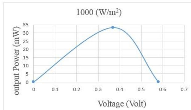
Figure 6: Maximum power of the used solar cell at 1000 (W/m<sup>2</sup>) intensity.
