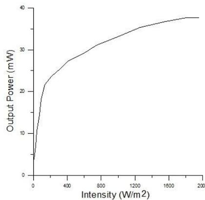
Figure 7: Variation of maximum output power from the solar cell with intensity.
