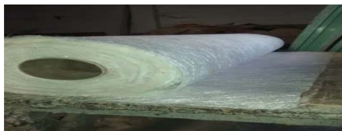
Fig-1 E-glass fiber with unidirectional fabrics
