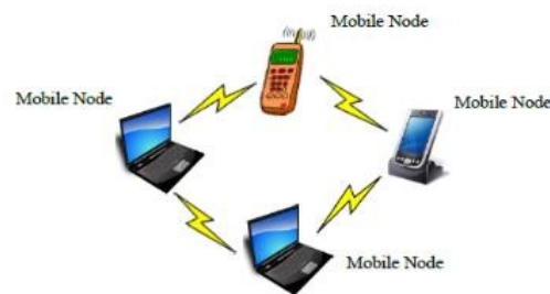
Figure 1: Structure of Mobile Ad Hoc Network (MANET) Source: A Survey on Routing Protocol and vulnerability in Mobile Ad-Hoc Network (MANET) Research Paper
