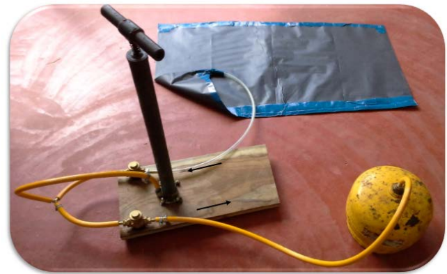
Figure 12: Complete system without pressure gauge
