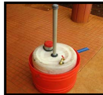
Figure 1: A domestic biogas digester (Mini Bio-gas plant using food waste, decomposable organic material and kitchen waste, n.d.)
