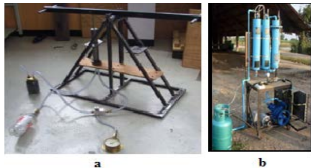
Figure 5: (a) Biogas bottling system (Nottingham) and (b) Biogas upgrading and bottling system in Thailand
