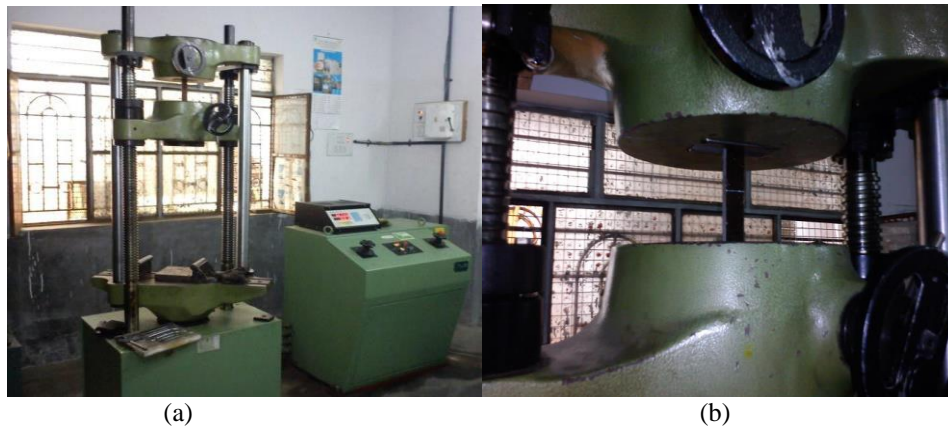
Fig.2 Universal Testing Machine. (a) Universal testing machine set up. (b) Specimen loaded in tension
