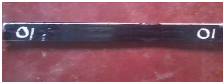
Fig. 1 Composite with 0% fiber prepared using Hand layup procedure
