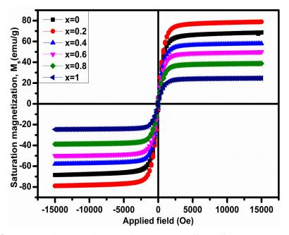
**Fig. 5.** The magnetic hysteresis loops of  $\text{Co}_{1-x}\text{Zn}_x\text{Fe}_2\text{O}_4$  ( $0 \le x \ge 1$ ) at room temperature.
