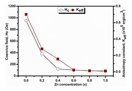
Fig. 8. Composition dependence of coercive field ( $H_c$ ) and effective magnetic anisotropy constant ( $K_{eff}$ ) of  $Co_{1-x}Zn_xFe_2O_4$  at room temperature.
