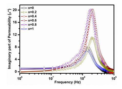
Fig 4b. Frequency variation of imaginary part of permeability of Co<sub>1-x</sub>Zn<sub>x</sub>Fe<sub>2</sub>O<sub>4</sub> (0≤x≤1).
