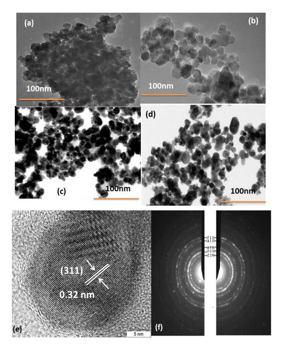
**Fig. 11.** TEM images of Ni<sub>0.4</sub>Zn<sub>0.2</sub>Mn<sub>0.4</sub>Fe<sub>2</sub>O<sub>4</sub>: (a) as-prepared powder, (b) sintered at 500°C, (c) 600°C, (d) 700°C, (e) High magnification HRTEM image of 700°C showing the (311) oriented lattice planes of Ni<sub>0.4</sub>Zn<sub>0.2</sub>Mn<sub>0.4</sub>Fe<sub>2</sub>O<sub>4</sub>, and (f) SAED pattern of d-spacing matched with XRD.
