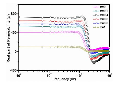
Fig 4a. Frequency variation of real part of permeability of Co<sub>1-x</sub>Zn<sub>x</sub>Fe<sub>2</sub>O<sub>4</sub> (0≤x≤1).
