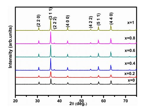
**Fig. 1**. XRD pattern of the  $Co_{1-x}Zn_xFe_2O_4$  ( $0 \le x \le 1$ ) nanoparticles synthesized at temperature 160°C for 15 min.
