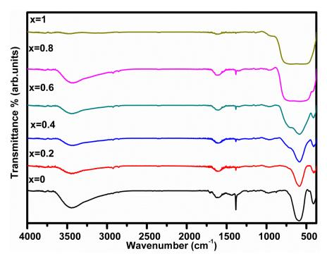
**Fig. 3.** FTIR spectra for as-prepared  $\text{Co}_{1-x}\text{Zn}_x\text{Fe}_2\text{O}_4$  ( $0 \le x \ge 1$ ).
