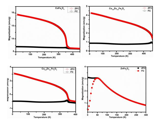
Fig. 6. Zero field cooled (ZFC) and field cooled (FC) curves of the Co<sub>1-x</sub>Zn<sub>x</sub>Fe<sub>2</sub>O<sub>4</sub> under an applied magnetic field of 50 Oe.
