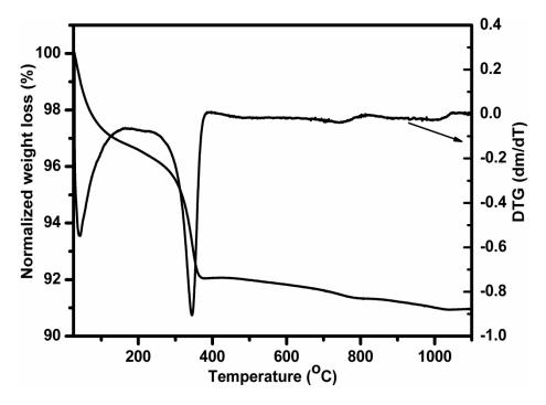
Fig. 9. TGA-DTG of  $Ni_{0.4}Zn_{0.2}Mn_{0.4}Fe_2O_4$  of dried gel.
