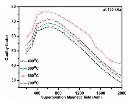
Fig. 14. Variations of Q-factor with superposition magnetic field.
