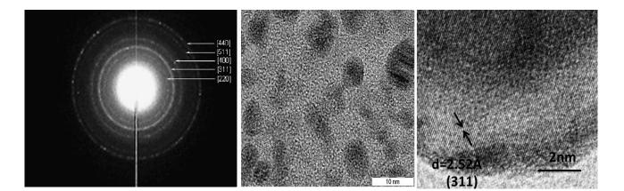
(a) (b) **Fig. 2** (a). SAED pattern of  $Co_{0,4}Zn_{0,6}Fe_2O_4$ . (b) High magnification HRTEM image of  $Co_{0,4}Zn_{0,6}Fe_2O_4$ showing the (311) oriented lattice planes.
