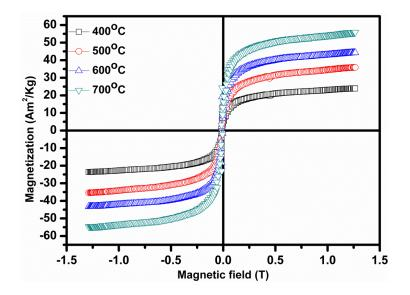
Fig. 12. Magnetic Hysteresis loops of Ni<sub>0.4</sub>Zn<sub>0.2</sub>Mn<sub>0.4</sub>Fe<sub>2</sub>O<sub>4</sub>
