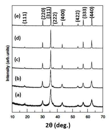
Fig. 10. XRD patterns of Ni<sub>0.4</sub>Zn<sub>0.2</sub>Mn<sub>0.4</sub>Fe<sub>2</sub>O<sub>4</sub> powder sintered at (a) 300 °C, (b) 400 °C, (c) 500 °C, (d) 600 °C, and (e) 700 °C.
