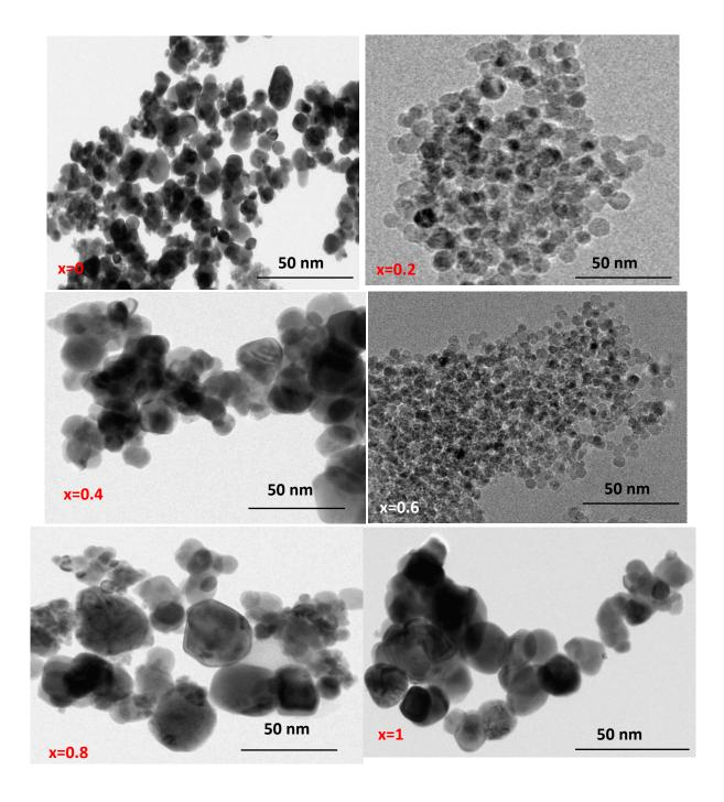
**Fig.2c.** TEM images of  $Co_{1-x}Zn_xFe_2O_4$  ( $0 \le x \le 1$ ) nanoparticles.
