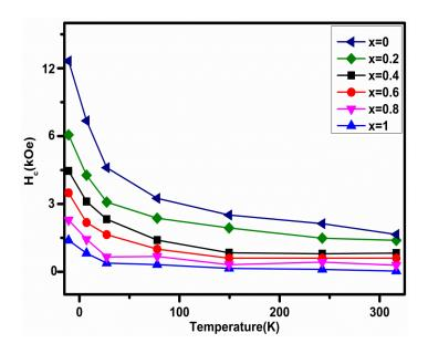
Fig. 7. Temperature dependence of the coercive field for  $Co_{1-x}Zn_xFe_2O_4$ .
