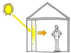
A trombe wall is system to trap heat from the sun and maintain apt temperatures and conditions for human comfort. This system contains a high wall of preferably dark colour and a glass panel a bit apart from the wall,
