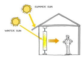
Sunspace beside the Trombe wall acts like a vented wall, heating the space through radiation as well as convection. Only the space between the wall and glass is big enough to move around in. These are basically used for direct gain of heat and would contain extra glazing in comparison to floor area. But loss of heat during night is not an issue as this room may be shut down during night.
