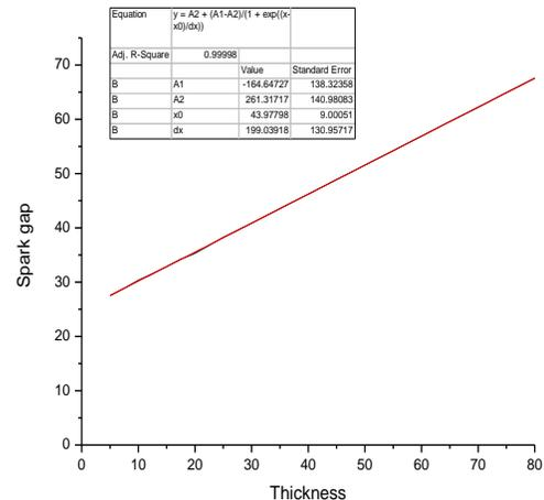
Figure 4: Effect of thickness on spark gap
