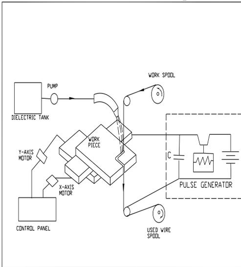
Figure 1: Schematic view of experimental set up
