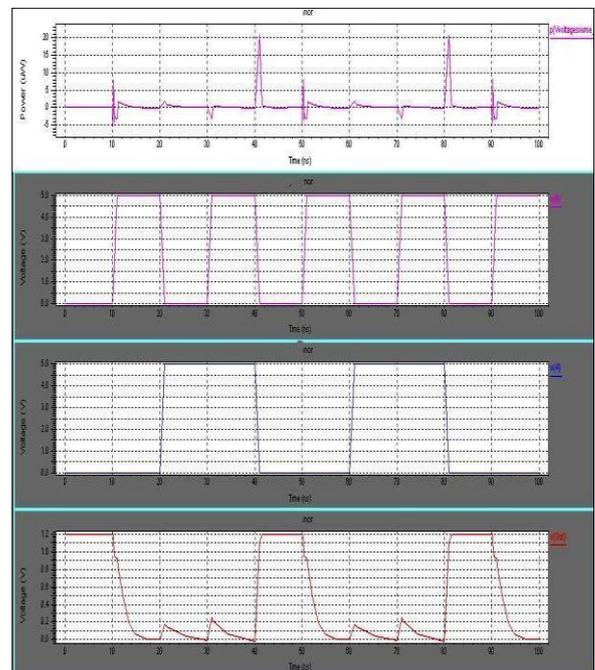
**Fig.10:Simulation waveforms of LCPMOS NOR**
