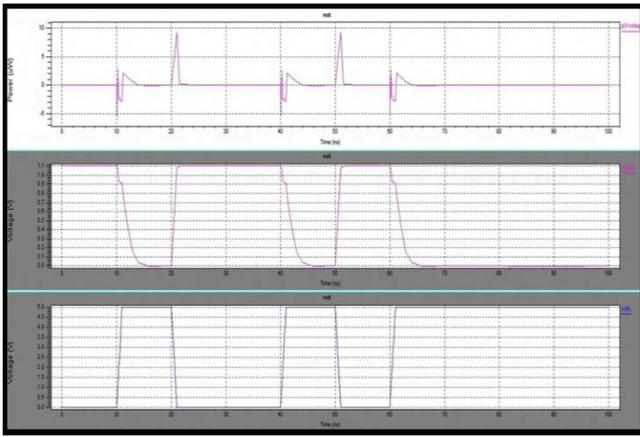
**Fig.6:Simulation waveforms of LCPMOS NOT**
