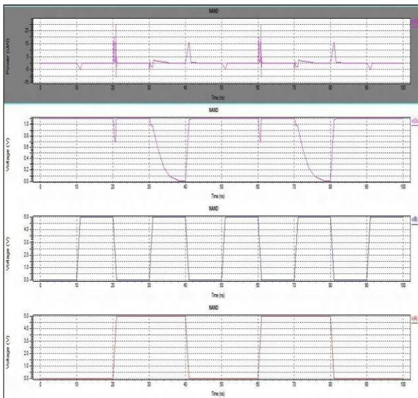
**Fig.8:Simulation waveforms of LCPMOS NAND**
