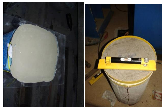
Fig- 5.2 Capping of Column Specimens
