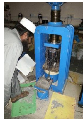
Fig 5.3 Under axial compression testing of column specimens
