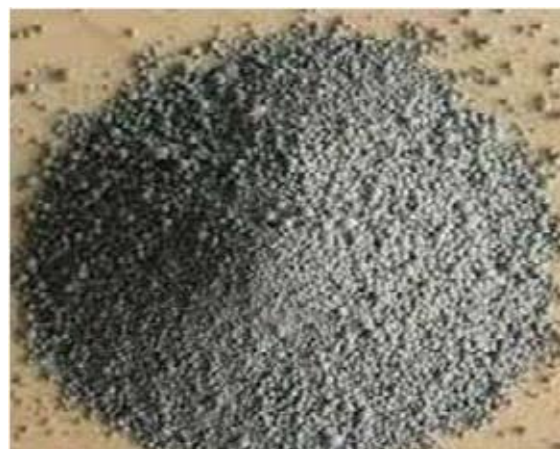
Fig 3. 1 Image of Micro-concrete
