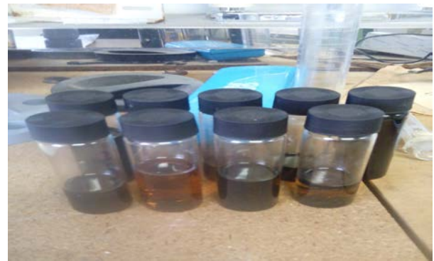
Figure 2: Liquid products with two immiscible layers. The gas produced during hydrogenation process was collected in gas collection bag. The gas in the collection bag was analyzed using GC – 14A gas chromatography and Agilent 3000 micro gas chromatography.
