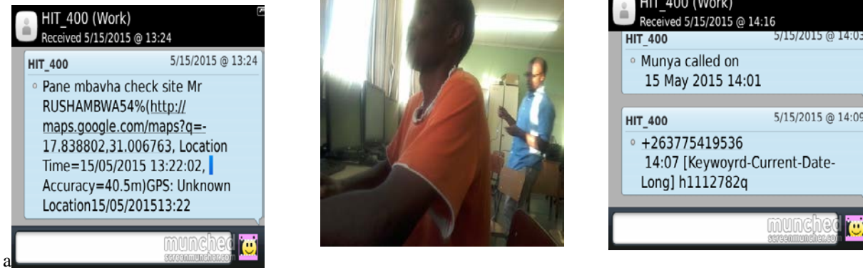
Figure (a). The message sent when motion is detected. (b). image taken when motion is detected. (c). call log SMS and encrypted message activation SMS
