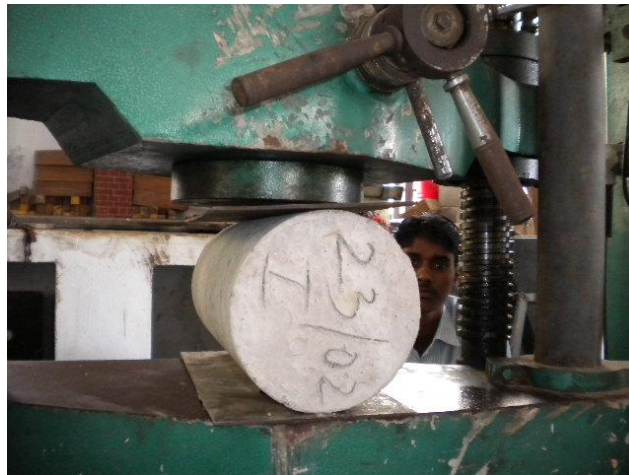
Figure-5. Split tensile strength testing on cylinders.
