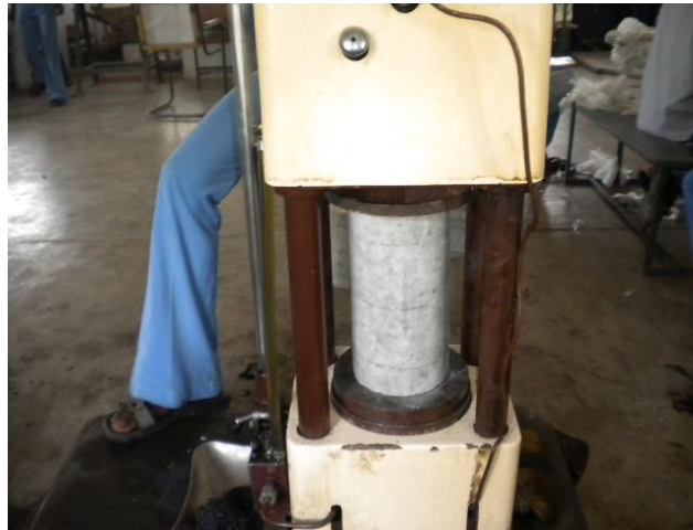
Figure-4. Compressive strength testing on cylinders.
