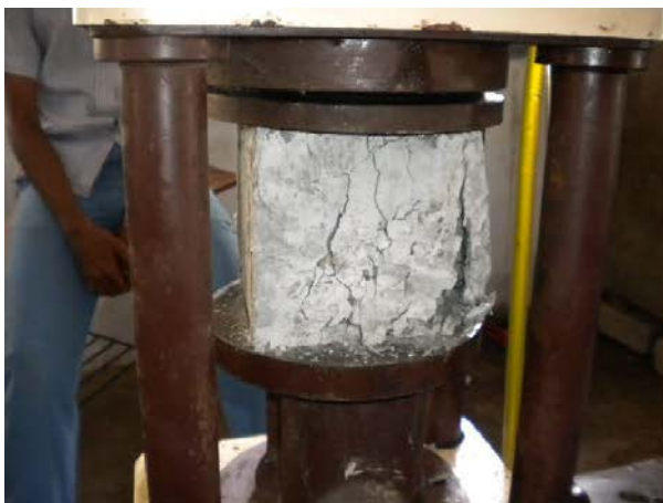
Figure-3. Compressive strength testing on cubes.
