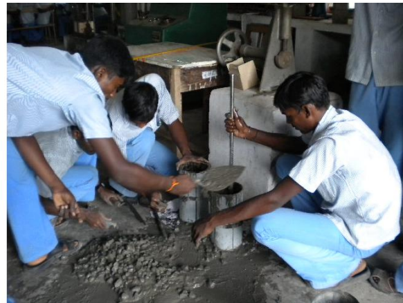
Figure-2. Casting of cylinders.
