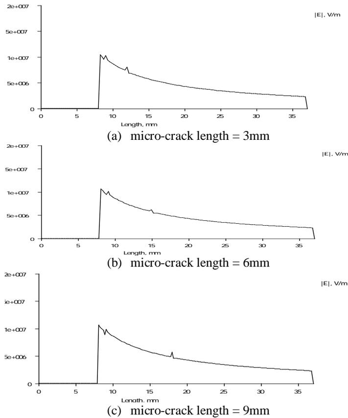
Figure 4. Lateral field distribution with micro-crack of radius  $30\mu\text{m}$ .
