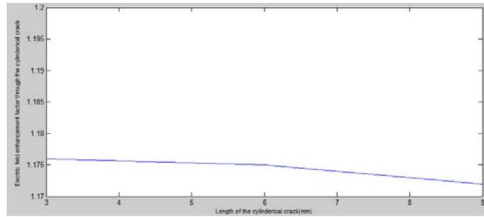
Figure 5. Enhancement field factor versus micro-crack length.
