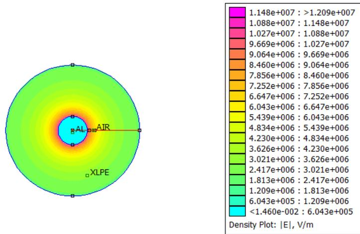
Figure 1. The electric field distribution inside a cross sectional area of a cable with the presence micro-crack.
