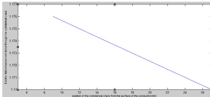
Figure 7. The enhancement field factor versus the distance between micro-crack and HV electrode.
