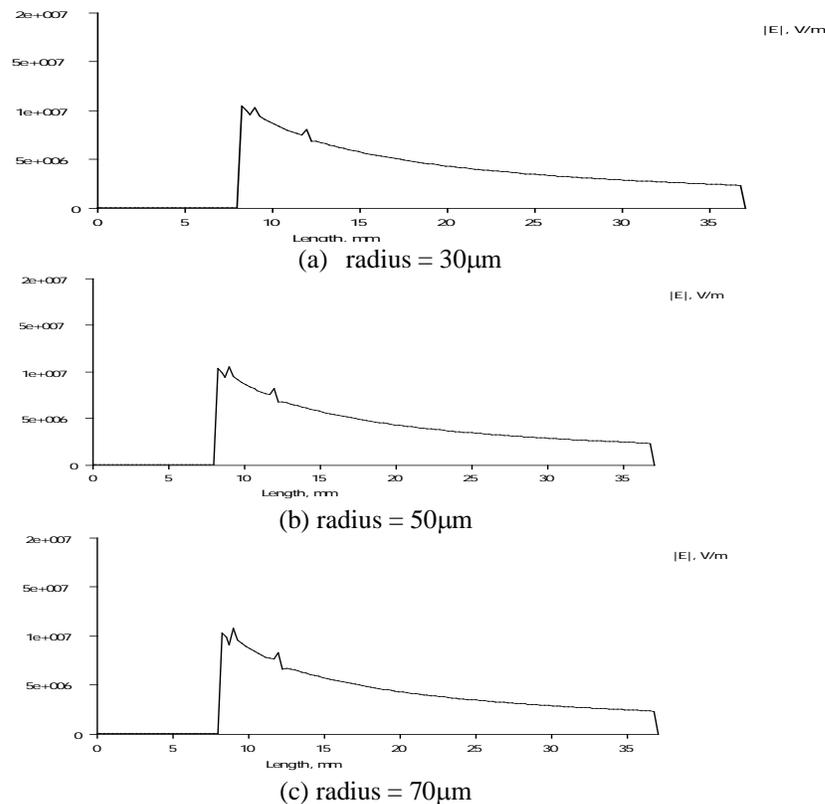
Figure 2. Lateral electrical field distribution with the presence of micro-crack.
