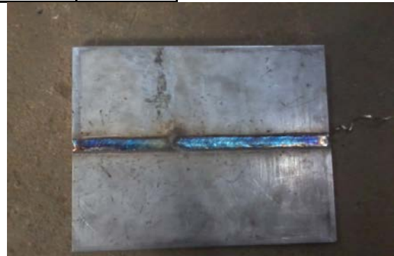
Fig.2: Fabricated Shielded metal arc weld (SMAW) metal
