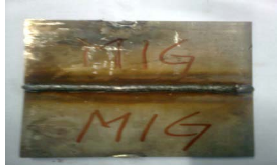
Fig.3: Fabricated Gas metal arc weld (GMAW) metal
