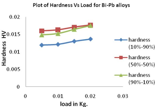
Figure 5 Graphs of Hardness vs. Load
