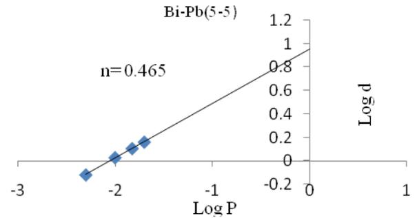
Figure 7 Plot of Log d vs. Log p for (5:5) Bi-Pb
