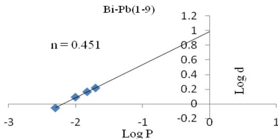
Figure 6 Plot of Log d vs. Log p for (1:9) Bi-Pb
