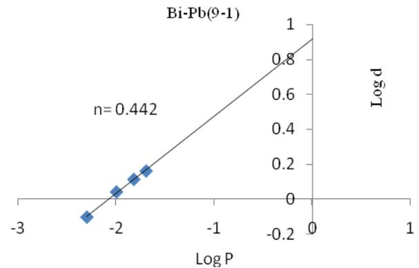
Fig. 8 Plot of Log d vs. Log p for (9:1) Bi-Pb
