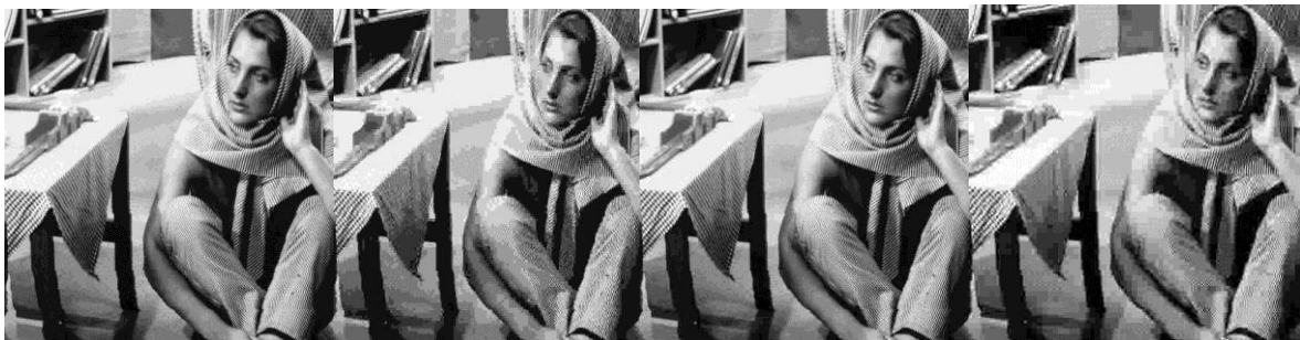
Block size 4×4 Block size 8×8 Block size 16×16 Block size 32×32 Fig.-08 (a) Minimum quantization matrix apply DCT & IDCT image reconstructed
