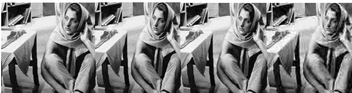
Block size 4×4 Block size 8×8 Block size 16×16 Block size 32×32 Fig.-08 (b) Woman (512×512) Maximum quantization matrix apply DCT & IDCT image reconstructed
