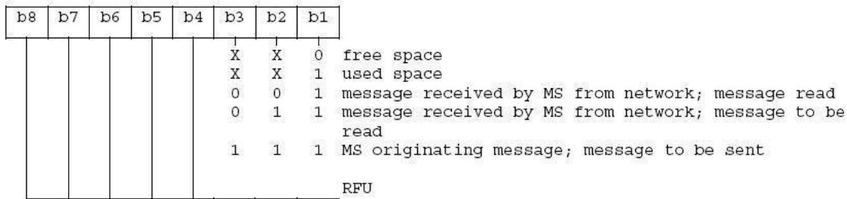
Figure 1: Structure of Status Byte
