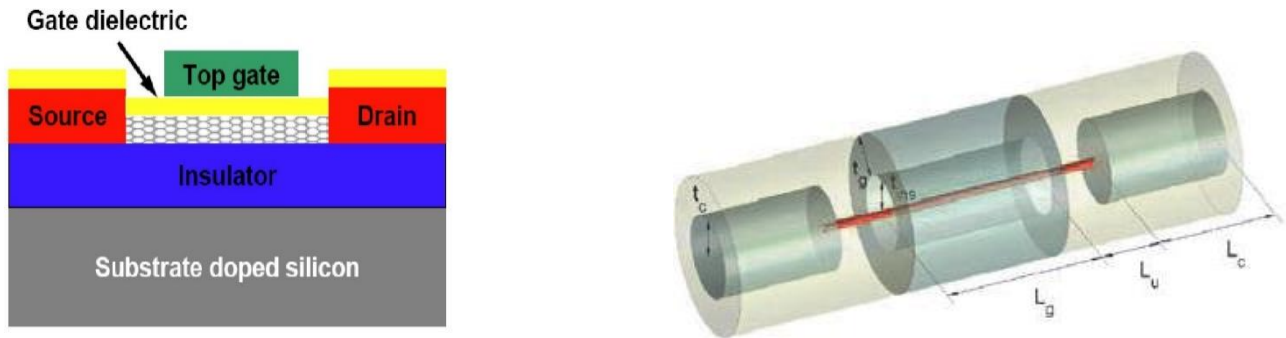
Figure 3: Carbon Nanotube Field Effect Transistor: Planar, Coaxial
