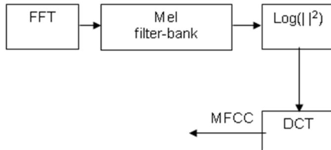
**Figure 1. Obtaining Mel cepstrum from windowed frames**
