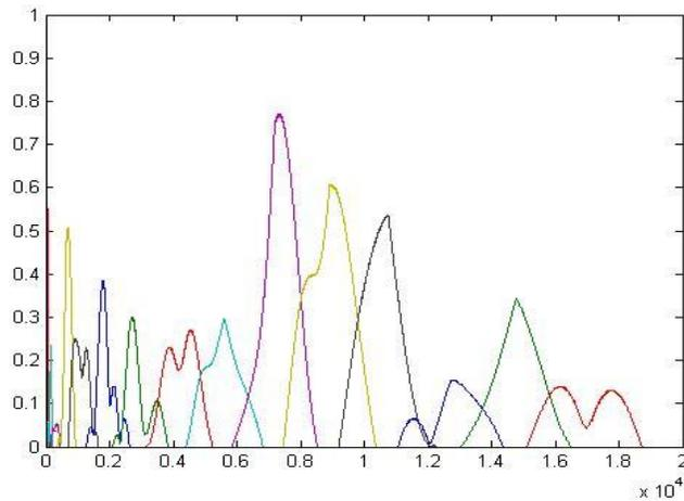
**Figure 5. Output of Mel scale filter bank**
