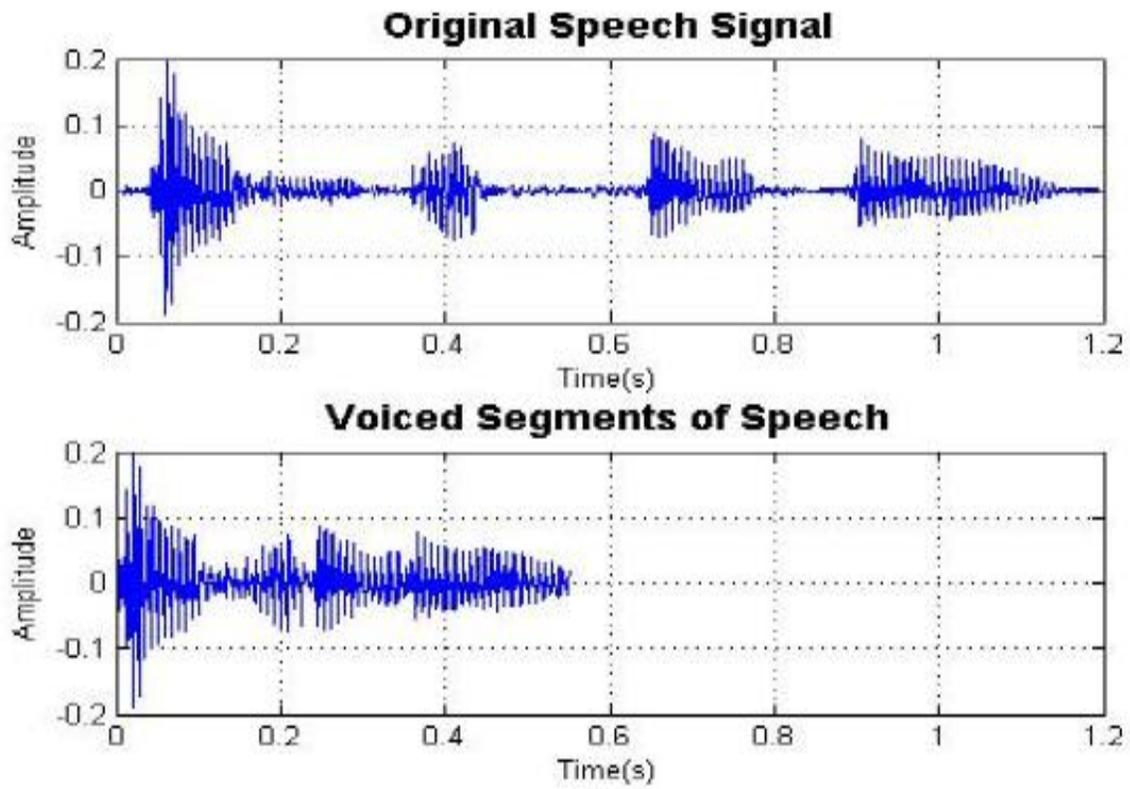
**Figure 4. Input and end point detected speech**
