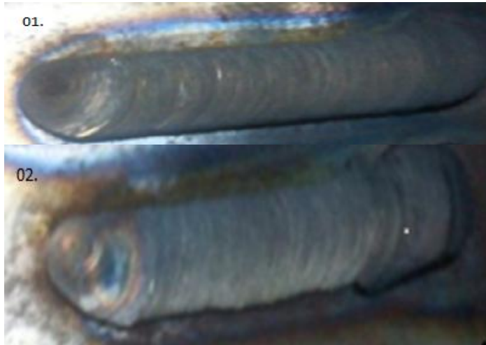
Fig. 4.5 Image of a M.S plate after friction surfacing using SS 304
