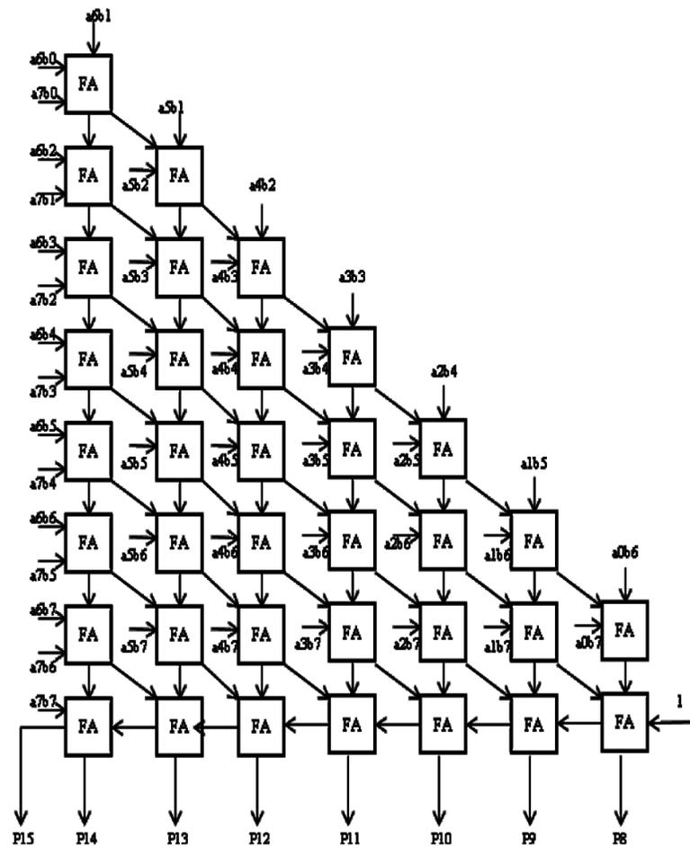
Fig.5 Architecture of truncated 8x8 multiplier.
