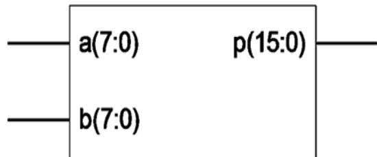
Fig.1 Block dig. of standard 8x8 multiplier
