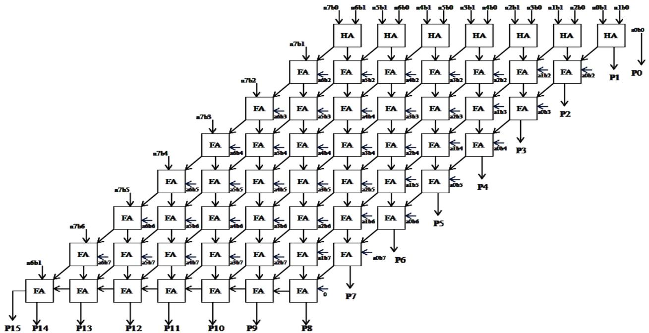
Fig.2 Architecture of 8x8 standard multiplier.
