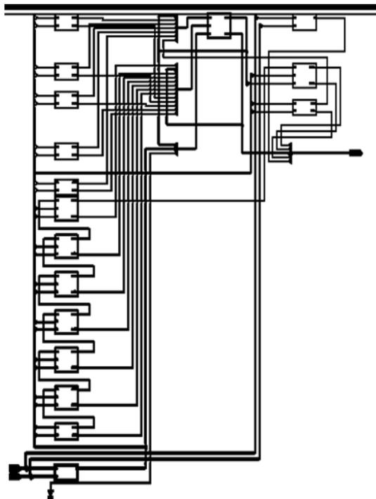
Fig.3 RTL schematic of standard 8x8 multiplier.
