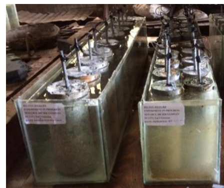
Figure 3:a) Schematic drawing of accelerated corrosion set up, b) Photo of the samples during experimentation
