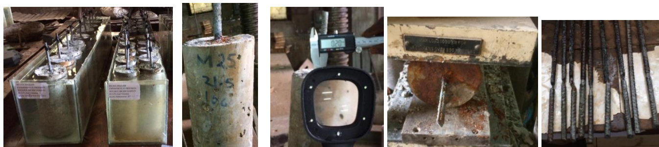
Figure 4: a) Samples during experimentation b) sample with 0.2mm longitudinal crack c) crack measurement d) recovering the corroded steel and e) cleaned rebar's for gravimetric weight loss measurement.
