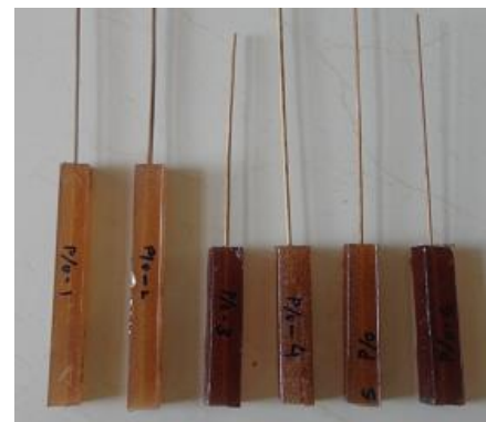
Figure 4: Specimens for single fiber pull-out test
