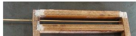
Figure 3: Mould for single fiber pull-out test
