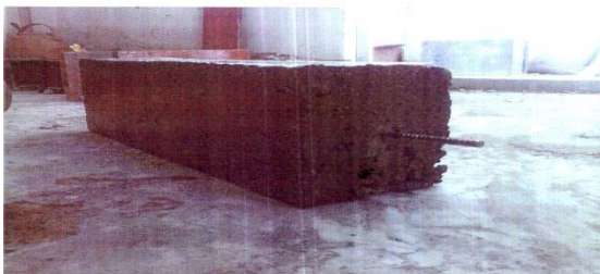
FIGURE:- Beam with sulphur coated steel bar
