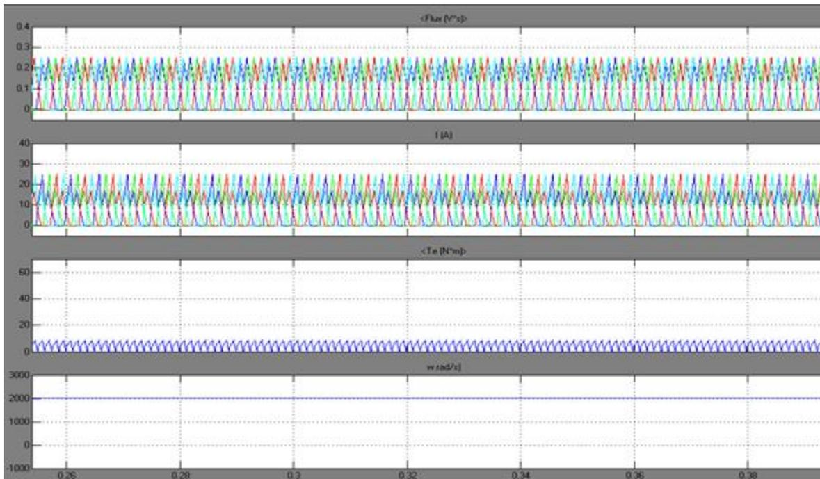
Figure 3: Steady State Waveforms of Flux, Current, Torque and Speed at healthy condition
