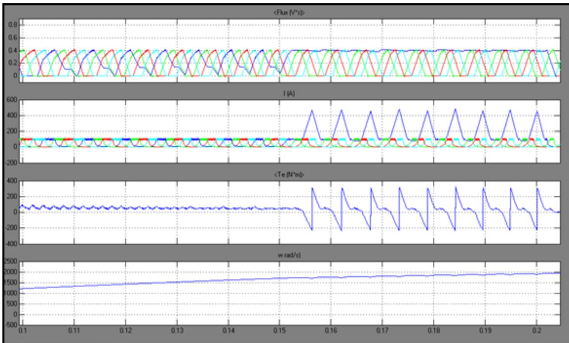
Figure 4: Waveforms of Flux, Current, Torque and Speed at inter turn short
