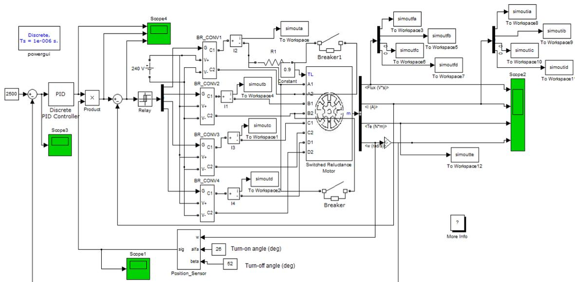
Fault detection in Current-controlled 8/6 Switched Reluctance Motor drive
