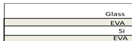
Fig 2: Cross section of a solar cell in a solar panel
