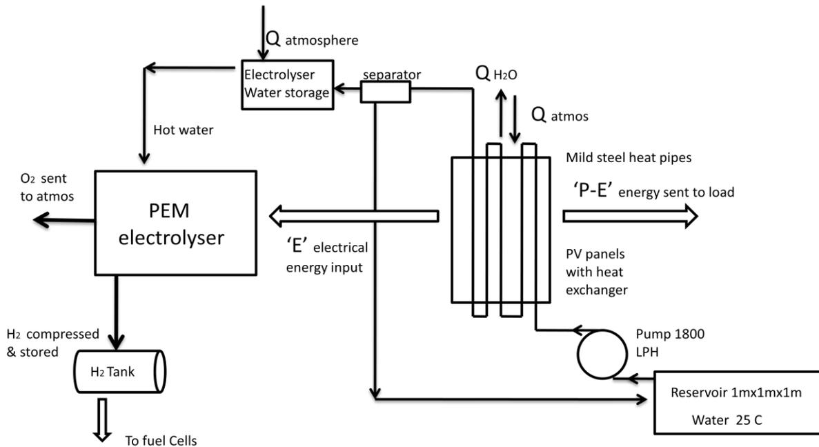
Fig 1: Schematic diagram of modified Solar Hydrogen Power System
