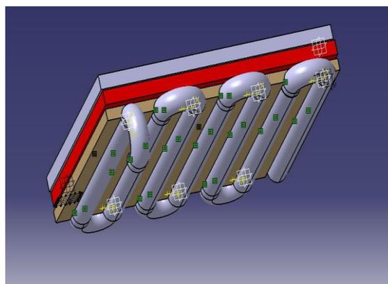
Fig 3: CAD design of heat exchanger pipes (Red colour: EVA layer, grey colour: cell layer)
