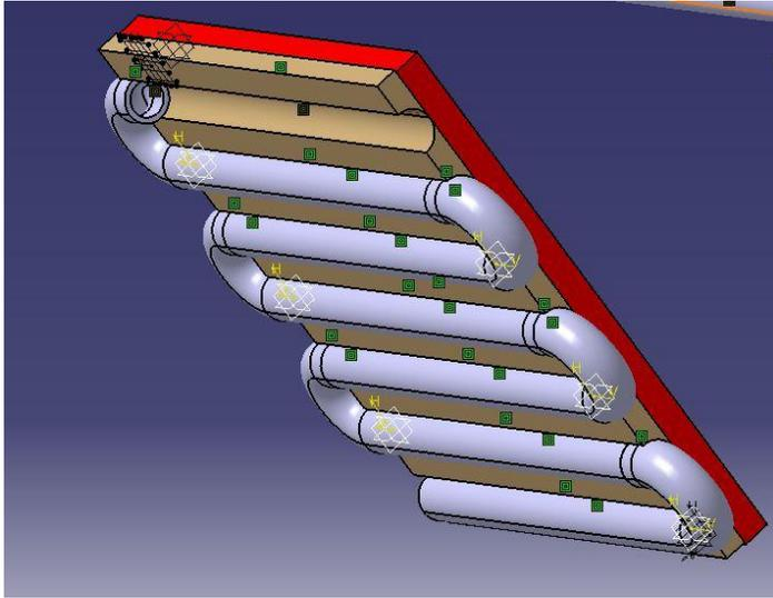
Fig 4: Arrangement of heat pipes in grooves
