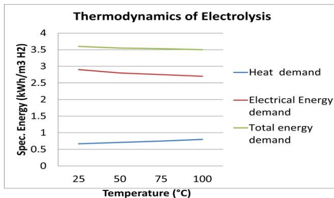
Fig 5: Thermodynamics of Electrolysis
