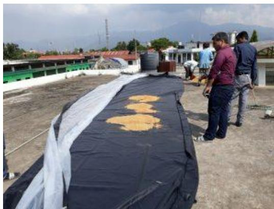
Fig. 1: Photographic view of assembling of Solar Bubble dryer (SBD) before start of experiment
