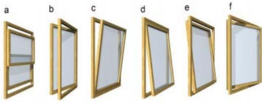
Figure 4: Window types examined by Grabe et al. (2014): a) double vertical slide window, b) turn window, c) bottom-hung window, d) awning window, e) horizontal pivot window, and f) vertical pivot window
