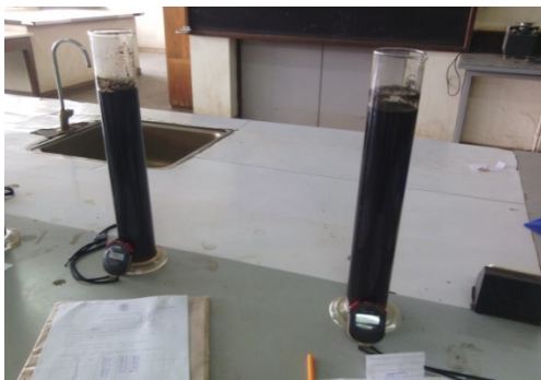
Plate 1. Hydrometer Analysis in progress
