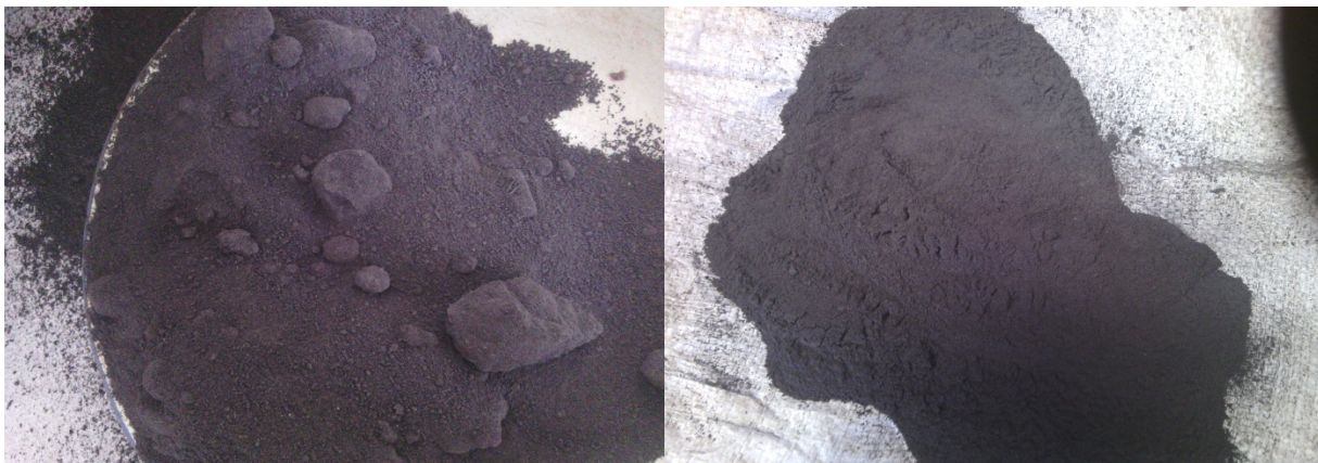
Plate 2. The SCBA, before and after grinding
