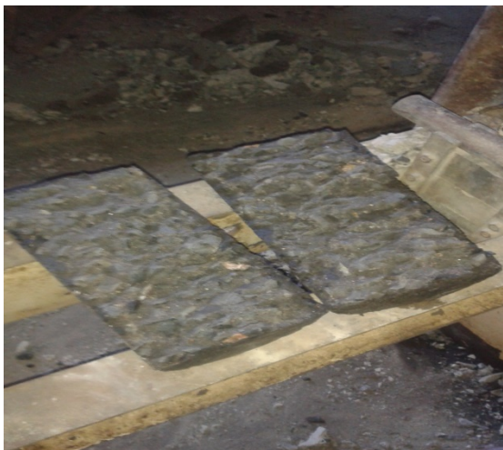
Plate 4. Failed tensile split cylinder sample
