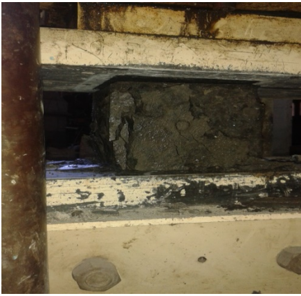
Plate 3. Failed compressive strength sample
